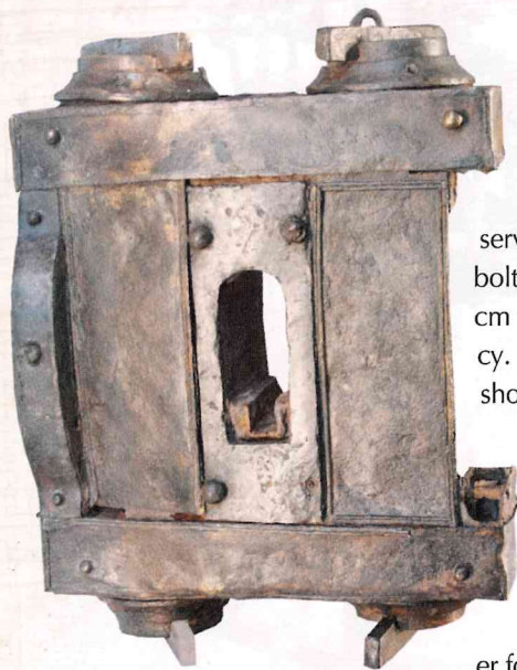
Tension frame of a small Roman torsion engine from the first century AD, found in Xanten, Germany.
